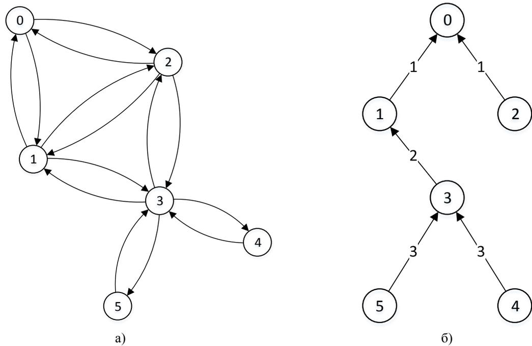
Figure 3 - Formation of the tree routing
